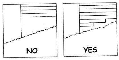
**FOUNDATIONS:** Visible foundation walls are limited to less than 18" vertically.
