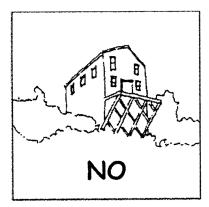
**DECKS**: Decks and their support structures must be carefully designed and detailed and be considered an integral part of the elevations. No X or knee bracing is allowed. Decks raised from 6-10 feet above the ground must be supported on columns at least  $7" \times 7"$ . Columns supporting decks over 10 feet above the ground must be least  $10" \times 10"$ . Columns may be boxed out to reach these required dimensions.
