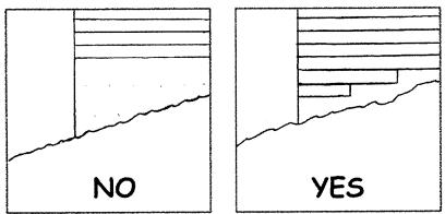
FOUNDATIONS: Visible foundation walls are limited to less than 18" vertically.
