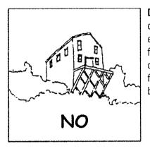
**DECKS**: Decks and their support structures must be carefully designed and detailed and be considered an integral part of the elevations. No X or knee bracing is allowed. Decks raised from 6-10 feet above the ground must be supported on columns at least 7" x 7". Columns supporting decks over 10 feet above the ground must be least 10" x 10". Columns may be boxed out to reach these required dimensions.
