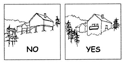
**DRIVEWAYS:** Driveway grades should be minimized. Designs that do not provide a reasonably level area just outside the garage may be rejected unless no feasible alternative exists. Driveways should be constructed so that all run-off water flows back to the street, or is collected with an area drain and piped the street or directly to the storm system.
