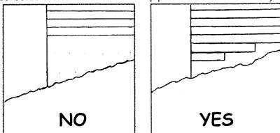
Amendment to CC&Rs of Sunridge First Addition - Page 2 of 5 Produced using RLID (www.rlid.org) on 08/06/2022 at 1:34 PM FOUNDATIONS: Visible foundation walls are limited to less than 18" vertically.
